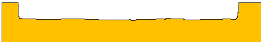
Figure 4: Shows the profile of a board which has been properly penetrated to 13cm.
