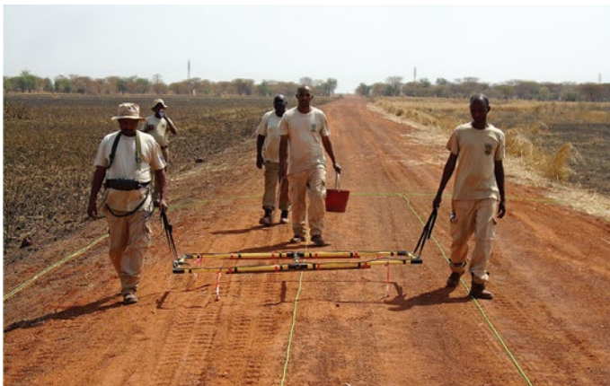
Quality control using Large Loop Metal Detector (LLMD) within the verified route in the Tishwin area (SDBZ)
