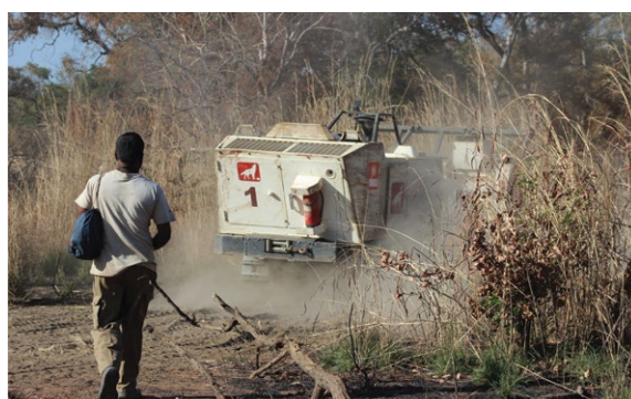
Minewolf operator remotely tracking the machine to the task site at JBVMM TS 11
